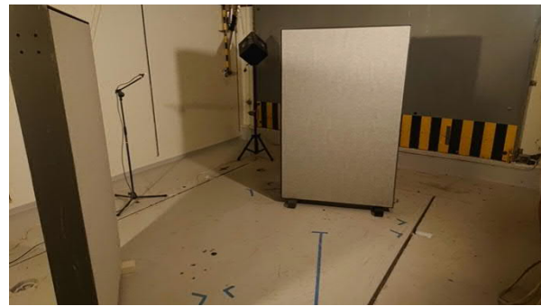
Figure 2: Two Lintex Unit 1800x1200 mm textile/textile, measured for sound absorption.
