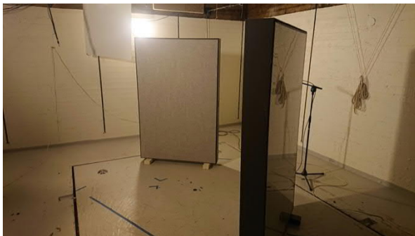
Figure 3: Two Lintex Unit 1800x1200 mm textile/glass, measured for sound absorption..
