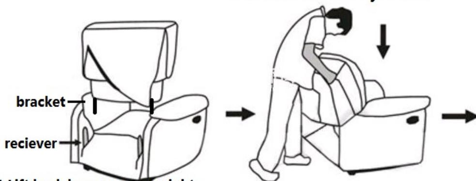
**1. Lift back loose cover upright, so metal brackets and reciever are aligned.**
