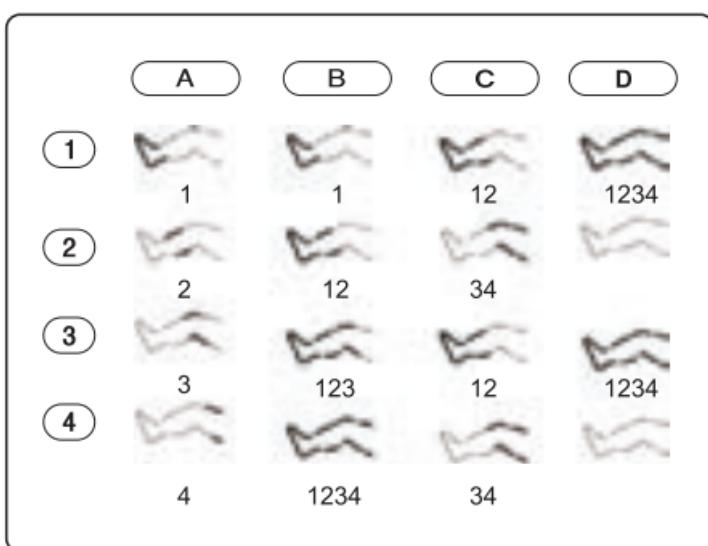
After starting the device, repeated pressing of the ON/OFF button changes the massage areas (1-2-3-4). Use the MODE button to change modes (A-B-C-D). The connection diagram of the modes and the principle of their operation are shown in the picture above. Using the TIMER button, we can freely set the sensor after which time the device will turn off automatically. The INTENSITY button changes the strength and intensity of the massage successively.
