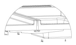
The crack between the two tops can be sealed with sealant. Be sure to clean the surface with a gentle household cleanser prior to sealing. Tops are made of ABS.
