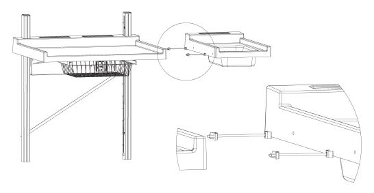
b) Make two ø8 mm holes in both top and sink as shown in drawing. Holes to be used with the fixing bolts.
